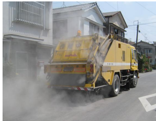
Fig. 5 A road sweeper conducting a clean-up operation. There are 96 vehicles for volcanic ash clean-up in Kagoshima city. (Photo courtesy of Kagoshima City Office)
